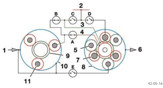
**Power Flow in 4th Gear:** Drive clutches A and E are engaged in 4th gear. Clutch A drives the sun gear 3 (4). Clutch E drives the planet carrier in the double planetary gear train. Together with the double planet carrier, the long planet gears and the short planet gears drive the internal gear 2 in the direction of engine rotation (gear up - ratio change).
